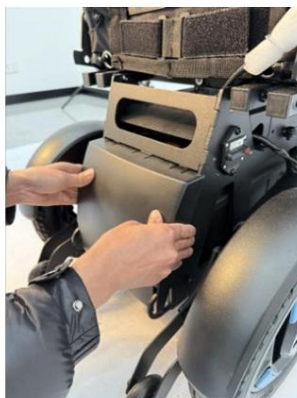
PAIGALDA AKUKATE (ALUMINE)
